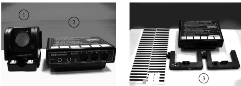
**Figure 1.** (1) Motion sensor, (2) Science Workshop 500 interface, (3) Photogates
